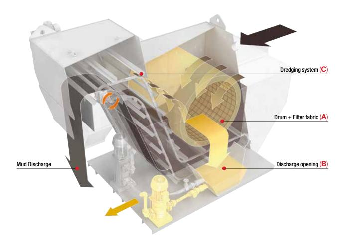
The Spring Compact working principle is divided in three main steps:
